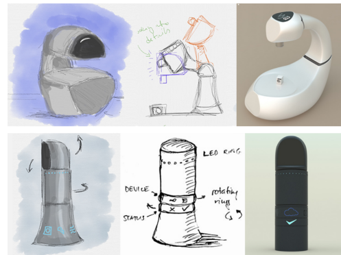
Fig. 2. Morphology sketches and high-fidelity 3D models of two concepts: Expressive Appliance (top) and Consumer Electronics (bottom).
