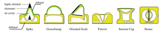
Fig. 4. Each Texture Unit is composed of an elastomer body, an embedded air cavity and optionally a haptic element. The TU deforms its surface under air inflation (green) and deflation (yellow).
