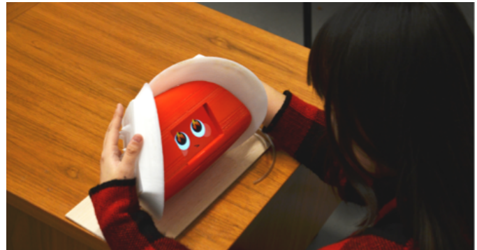
Fig. 1. A social robot prototype combining facial expressions and a texture-changing skin. During the interaction, the user makes eye contact with the screen face and puts their palms on the sides of the robot to touch the actuated textures.
