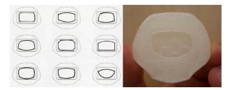
Fig. 4. Screen faceplate designs allowed us to vary the appearance of the robot using one design.
