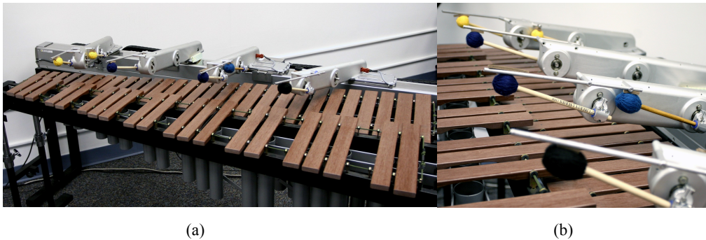
Figure 3. Overall (a) and detail view (b) of the robotic marimba player Shimon . Four arms share a voice-coil actuated rail. Two rotational solenoids per arm activate mallets of varying firmness.
