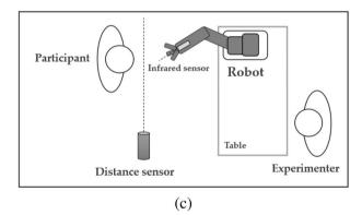
**Fig. 3** Experimental Setup: Video frames of an actor handing over an object to the robot, used in the video study: **a** "Standing" posture **b** "Sitting" posture **c** Diagram of the setup for the in-person study
