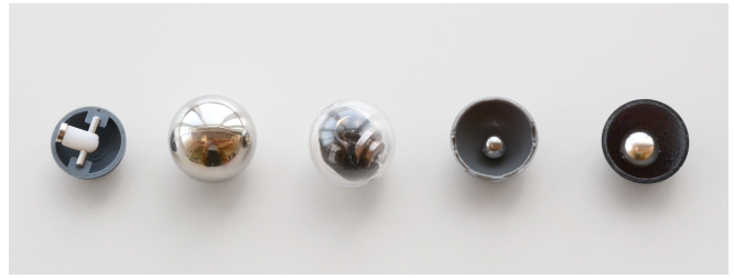
Fig. 4. The various rolling balls designed and tested with the Greeting Machine, spanning a variety of external materials, internal rolling constraints, and ferromagnetic components.
