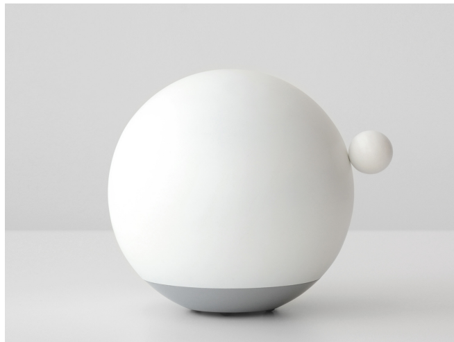
Fig. 1. The Greeting Machine, a low-DoF robotic object designed for opening encounters, in the form of an abstract ball rolling on a dome.
